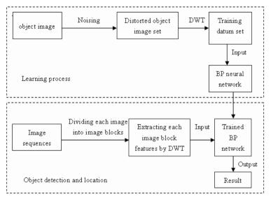
Fig. 1. Location and track an object in image sequences by BP networks
