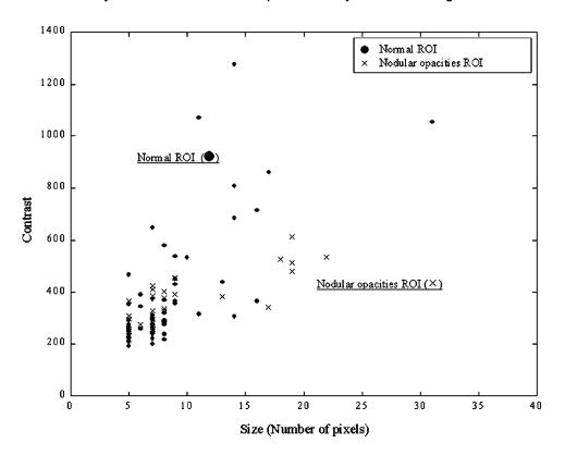
Fig. 4. The relationship between the size and contrast of initial candidates for nodular components in two ROIs selected for normal and nodular opacities. The initial candidates for the nodular component with the contrast above 700 were removed as small circular blood vessels.
