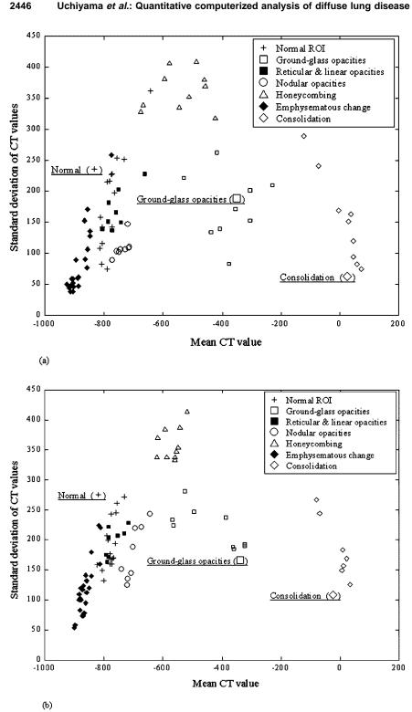
Fig. 7. A comparison of two distributions of physical measures obtained from (a) small ROIs (32×32) and (b) large ROIs (96×96).
